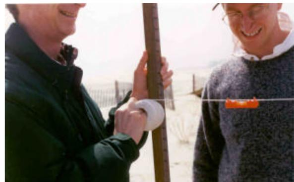
Figure 1-5: The line level is “level” and the string is used to determine the elevation reading on the long rod.
