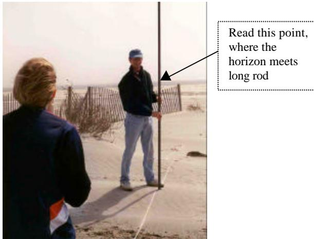
Figure 1-3: The woman is sighting a line from the short rod to the long rod, directly towards the horizon. The arrow indicates where the man will read the measurement.
