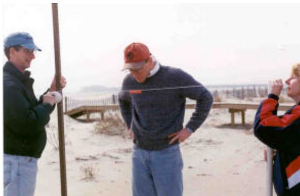
Figure 1-4: Using the line level to measure elevation change when the horizon is not in view.
