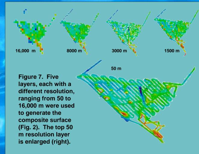
Figure 7. Five layers, each with a different resolution, ranging from 50 to 16,000 m were used to generate the composite surface (Fig. 2). The top 50 m resolution layer is enlarged (right).
