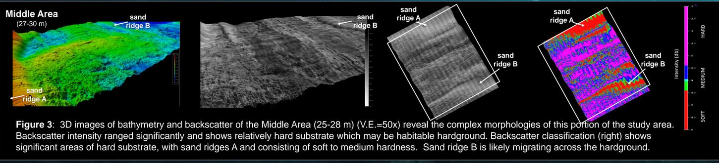
**Figure 3:** 3D images of bathymetry and backscatter of the Middle Area (25-28 m) (V.E.=50x) reveal the complex morphologies of this portion of the study area. Backscatter intensity ranged significantly and shows relatively hard substrate which may be habitable hardground. Backscatter classification (right) shows significant areas of hard substrate, with sand ridges A and B consisting of soft to medium hardness. Sand ridge B is likely migrating across the hardground.
