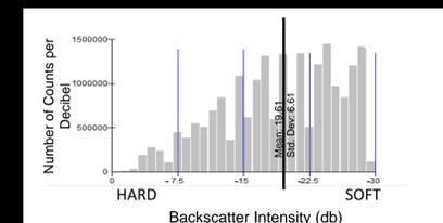
**Figure 5:** Frequency of the backscatter intensities for the study area. Relatively hard substrate occurs between 0 and -15 db. The majority of the study area is relatively soft substrate with backscatter intensity of -15 to -20 db. Intensity was then used to classify substrate, shown in Figs. 2, 3, 4, and 6.
