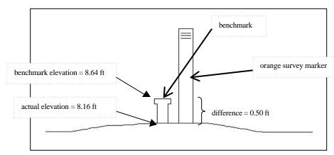
Figure 1-2: Find the vertical difference between the benchmark elevation and the land surface to determine the land surface elevation. In this example, subtracting the vertical difference (0.50 ft) from the benchmark elevation (8.64 ft) results in an actual elevation of 8.16 ft.
