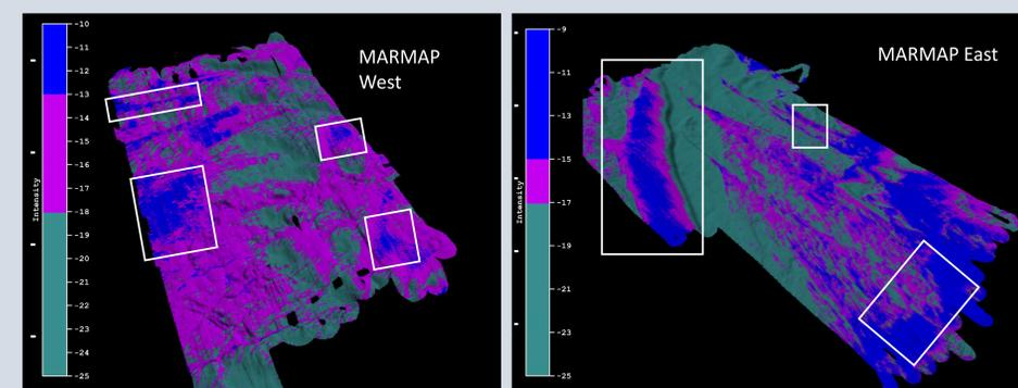
**FIGURE 5.** Ideal habitat areas indicated for MARMAP West and East, based on bathymetry and classified backscatter data.
